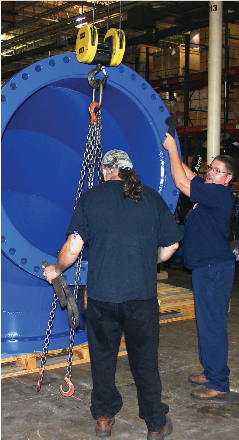
State of the art designs such as this 54" restrained elbow for ductile iron pipe
