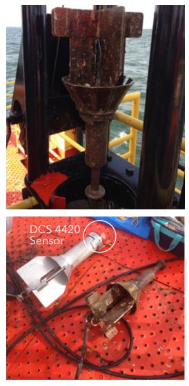
Fig3: Aanderaa DCS system from Xylem (LEFT) lying next to the previously installed EM sensor (RIGHT)
