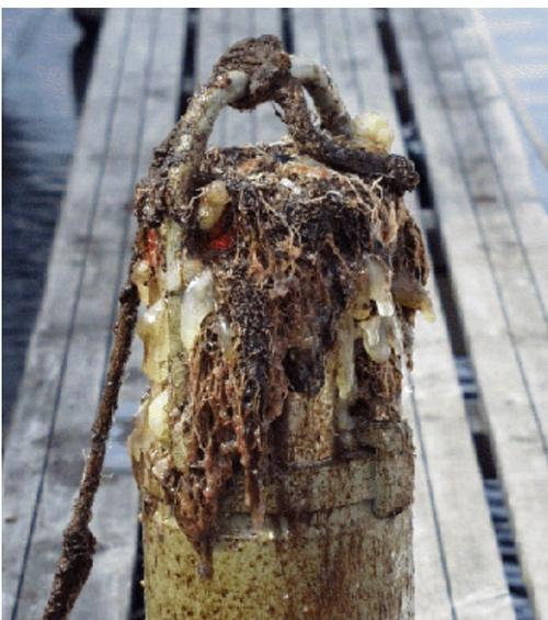
Fouling consisting of calcareous organisms (e.g. barnacles), can be dissolved by dipping the sensor/instrument in a weak acid solution (e.g. 7% Vinegar).
