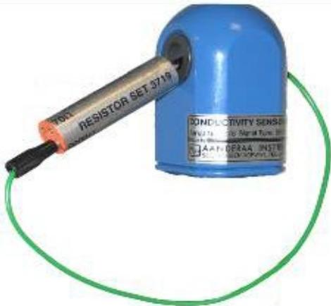
**Figure 7-2: Conductivity Sensor with resistor set**
