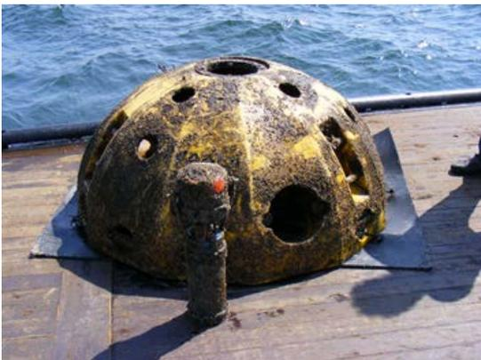
Fig. 4: RDCP-600 with bottom frame on dock during 6 months service and exchange of broken cable, dredged off.
