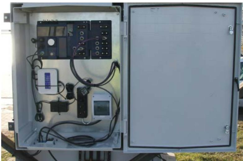
Fig. 6C: Cabinet with Aanderaa SmartGuard, Globe Star III GPRS modem and power supply
