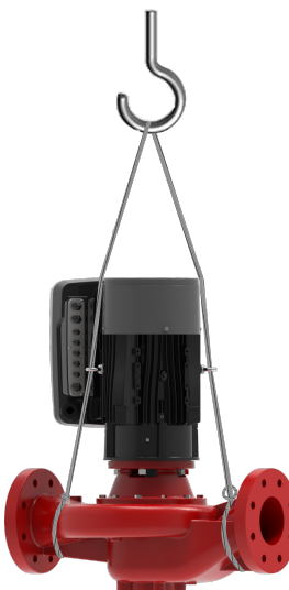
Lifting option 2: Sling around pump flanges and use motor eyelets as guides to maintain balance while lifting.
