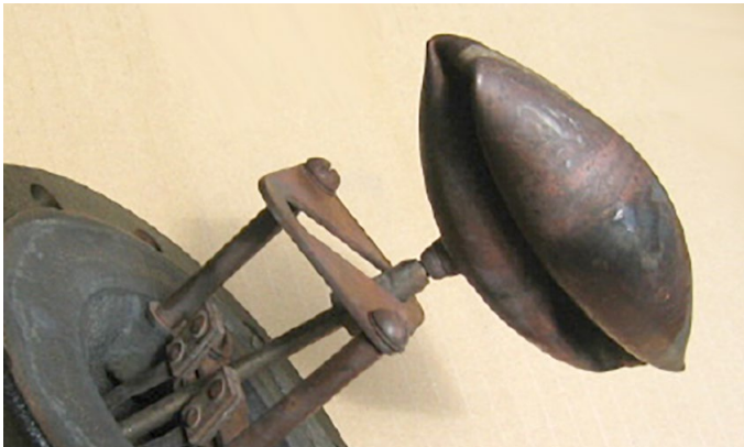
McDonnell & Miller float destroyed by water hammer
