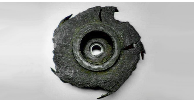
Impeller destroyed by cavitation
