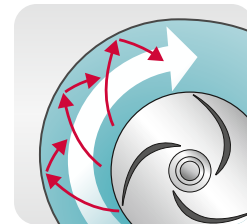
Standard impeller slams solids into the volute.
