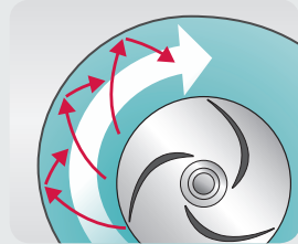
Standard impeller slams solids into the volute.
