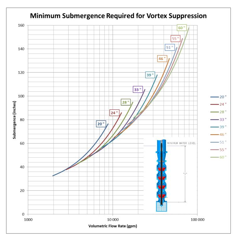
Figure 2 - Minimum Submergence Curves - Diameters 20" - 60" - Imperial Units
