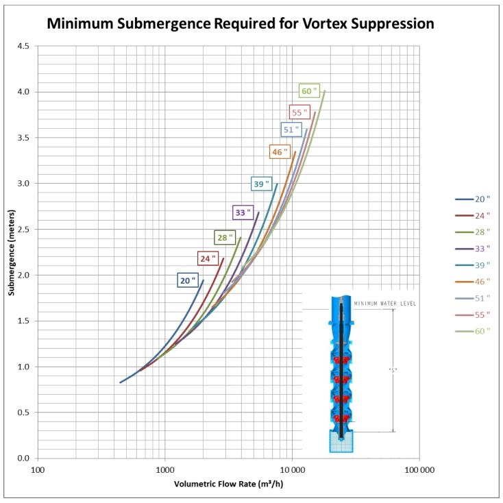
Figure 4 - Minimum Submergence - Diameters 20" - 60" - SI Units
