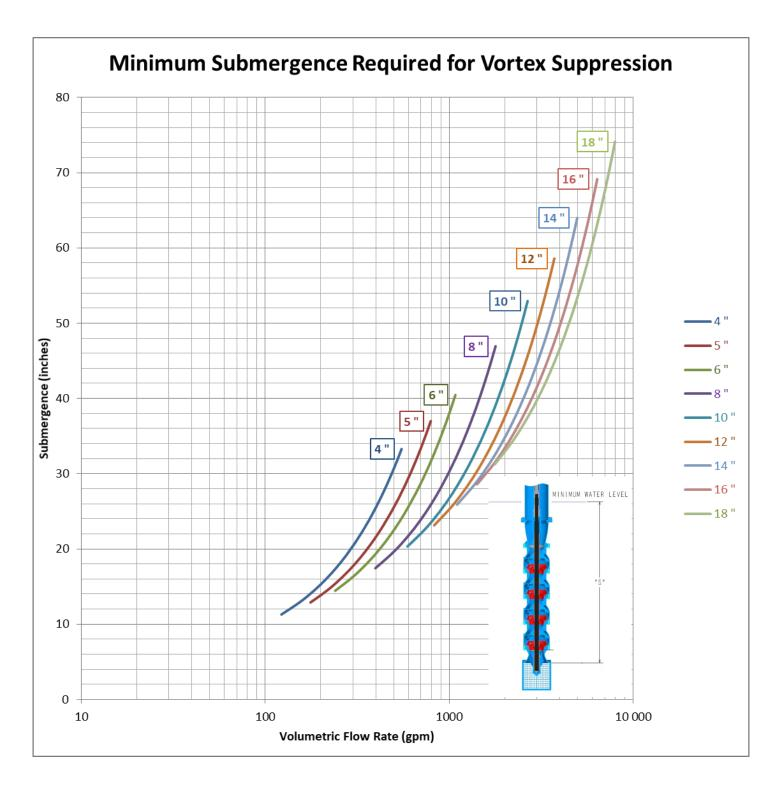
Figure 1 - Minimum Submergence Curves - Diameters 4" - 18" – Imperial Units
