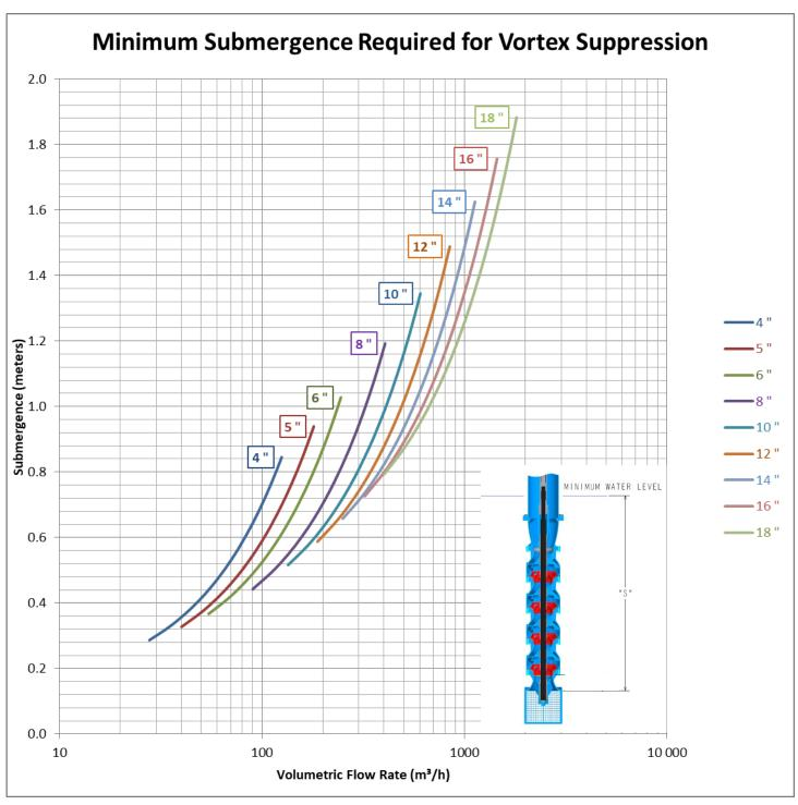
Figure 3 - Minimum Submergence Curves - Diameters 4" - 18" - SI Units
