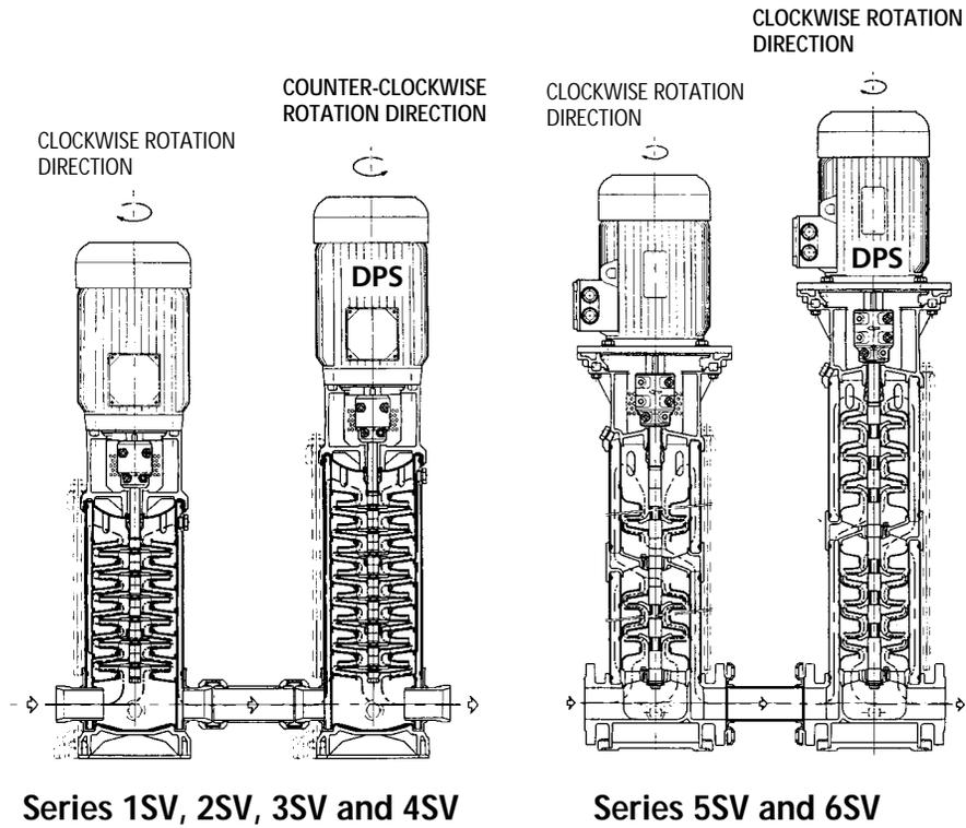
Refer to the above diagram for proper pump installation detailing flow direction and motor rotation. All DPS units will be properly tagged with flow direction and motor rotation labels. Please ignore all cast direction arrows. Note that the DPS pump is the second unit after the lead SSV unit.
