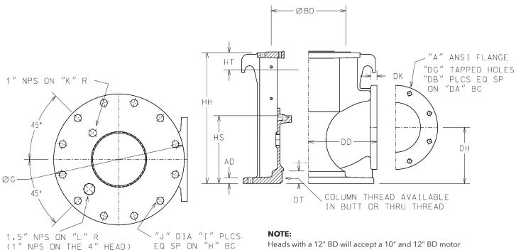
Heads with a 12" BD will accept a 10" and 12" BD motor Heads with a 16.5" BD will accept a 20" and 24.5" BD motor Heads with a 20" BD will accept a 16.5" and 24.5" BD motor Heads with a 24.5" BD will accept a 16.5" and 20" BD motor
