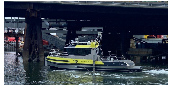
Autonomous vessel piloted by the Sea Machines SM300 autonomous system.
