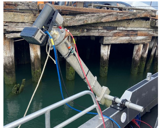
Survey data collected by a Teledyne T20 MBES and Applanix POS MV installed on the vessel.
