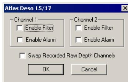
**Enable Filter:** If an error has been detected, depth is changed to 0.
