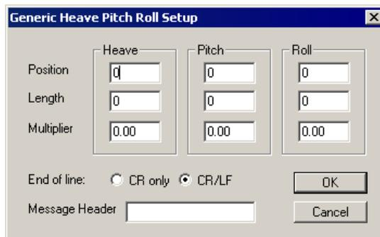
**Position** determines the character position in the device output string for each value.
