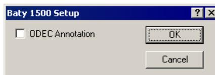
**ODEC Annotation:** sends \$GPANN string to both device window and serial port.
