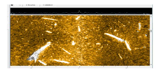
The nadir dampening options allow you to lower the brightness of just the nadir, allowing it to blend better with the rest of the data.
