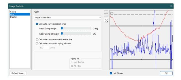
Additionally, this new gain option allows you to dampen the nadir. In this dataset, you may notice the center of the waterfall is consistently brighter than the edges:
