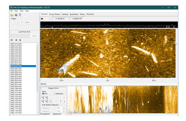
There's a new gain option that works great with backscatter data as well. It's a modification of our Angle Varied Gain that uses data across all lines to create a gain curve.
