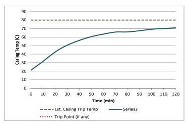
Tested @ ambient temp of 70F (21.1C) @ max run pressure Trip point shown is casing temp at time of TCO trip
