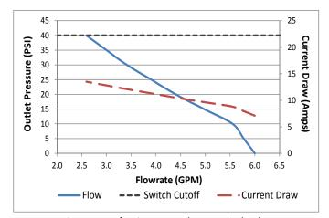
Representative curve of unit operated at nominal voltage Performance will vary somewhat unit to unit Switch cut-off represents the point on the flowcurve at which the integrated pressure switch will turn off the pump
