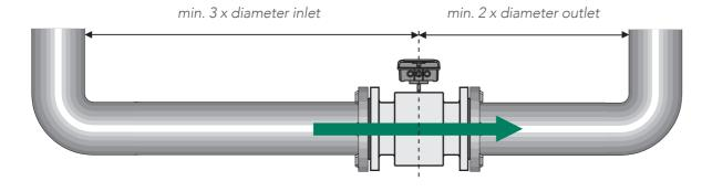
Special design allows using short build-in construction still providing very accurate flow measurement even at one pipe diameter of straight pipe upstream and one pipe diameter of straight pipe downstream from the center of the flow sensor.
