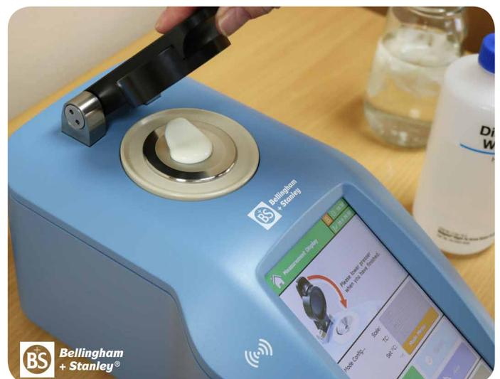
Fig. 7b: Latest RFM340-T refractometers are capable of measuring to 3 decimal places Brix and can measure the total dissolved solids of nonhomogeneous samples such as yoghurt drinks with ease. The new touchscreen interface and clever software takes refractometry to a new level unsurpassed by other manufacturers.
