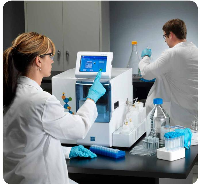
Fig. 9: The YSI 2900 Series Analyser can not only differentiate specific sugars in a diverse foodstuff, it can also be used to monitor ethanol build-up in fruit juices and fresh fruit.
