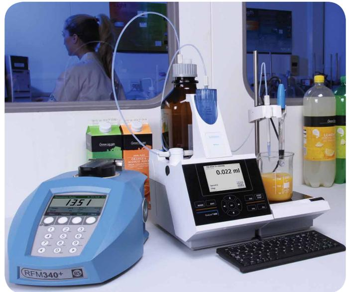
Fig. 1: The popular RFM340+ Series Peltier temperature controlled refractometer (left) used to control Brix in the factory or laboratory next to a TitroLine 7000 auto-titrator (right) for controlling acids and diet beverage concentrations
