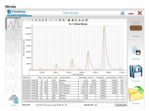
**Figure 3.** Calibration Series for Determination of Nitrate and Nitrite in Milk and Milk Products Using Cadmium Reduction and FIA with In-line Dialysis
