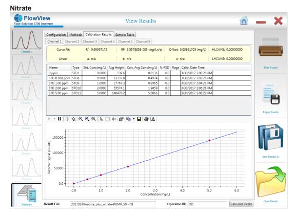
**Figure 4.** Calibration Curve and Statistics for Determination of Nitrate and Nitrite in Milk and Milk Products Using Cadmium Reduction and FIA with In-line Dialysis
