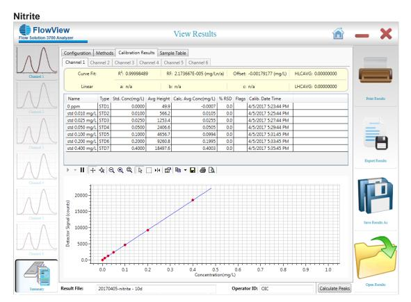
Figure 6. Calibration Curve and Statistics
