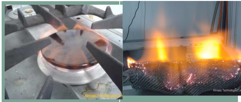
Figure 6: laboratory experiments of hydrogen combustion using standard atmospheric burners; primary air inlet blocked off using proprietary paste (left) and primary air inlet blocked off and wrapped in metal fibre blanket (right)
