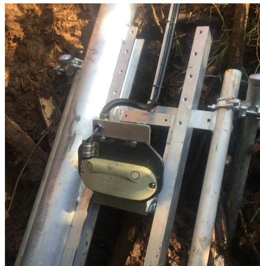
Fig. 3. Sliding Rail and Mount
