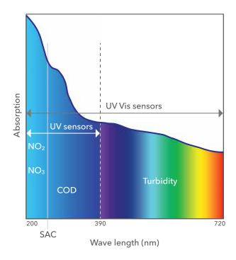
**Figure 1.** Ultraviolet and visible spectrum of light from 200-720 nm. Nitrate and nitrate primarily absorb UV light from 200-250nm and organic molecules from 250-350nm. Turbidity absorbs light from 380-720nm.
