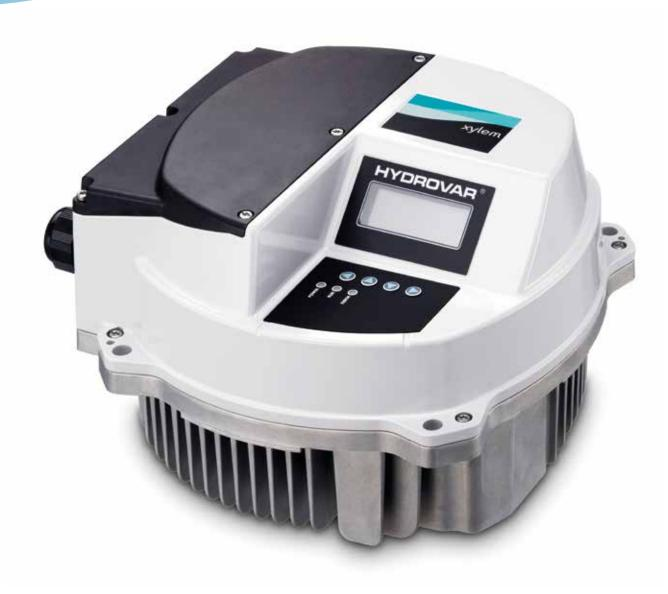
Retrofiitting the 'plug and play' HYDROVAR units to a fixed speed booster set not only eliminates the need for a control panel but also introduces a soft start function, that when combined with the benefits of running a pump at a variable speed, can prolong the life of the pump and the water system. By reducing the in-rush current when the pump is turned on, parts such as motor bearings and pipe fittings are protected from hydraulic shock that can cause cavitation and breakdown.
