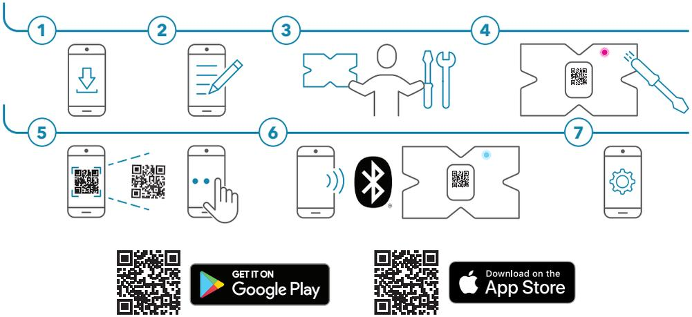
1 Download the optimize app 2 Complete user registration 3 Physically install your sensor (see side 2) 4 Wake up your sensor by placing the supplied magnet over the Bluetooth® icon until the LED blinks pink\* 5 Scan your sensor QR code OR enter the S/N manually 6 The sensor and your device should now be paired (indicated by a blue LED) 7 Create your asset profile and automatically begin monitoring
