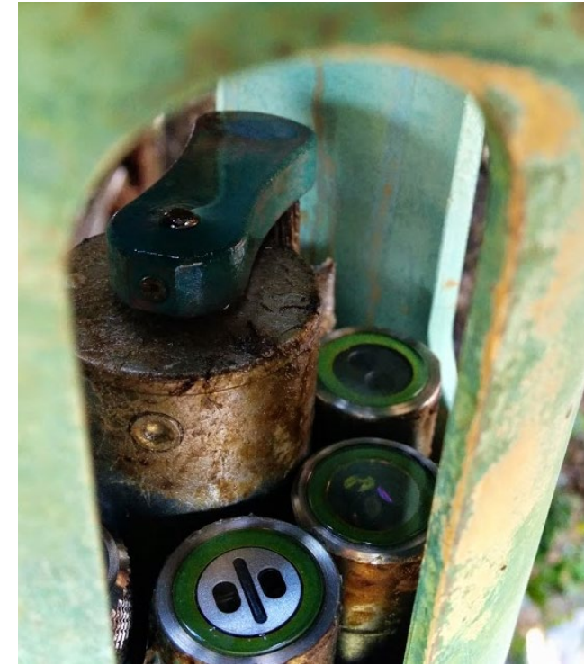
Post-deployment Wiped sensing area free of biofouling.
