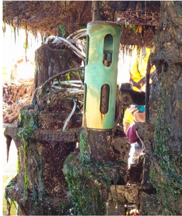
Post-deployment Heavy fouling prevented by copper sensor guard.
