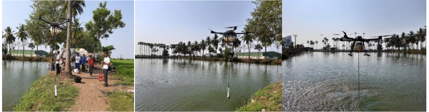
Functional Demonstration of Drone mounted with CTD sensor & other instrumentation payload for Ocean Data Collections
