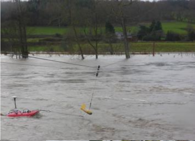
Torrent Board carrying M9 RiverSurveyor on River Tyne
