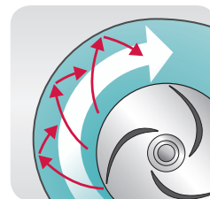
Standard impeller slams solids into the volute.
