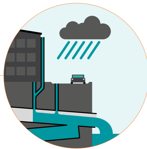
Combined Sewer Overflow (CSO)
