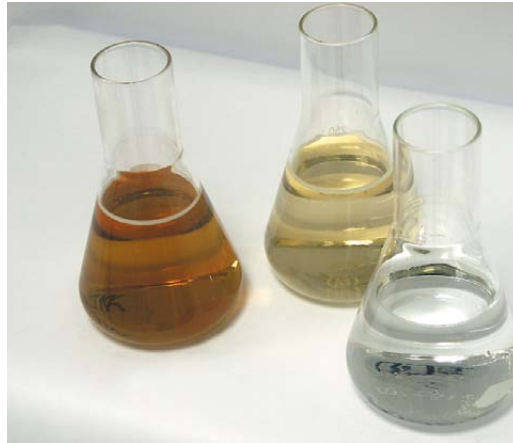
Fig. 8: Colour elimination with ozone
