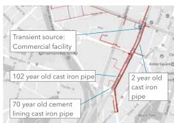
**Pipelines at risk of failure** identified based on exposure to transient pressure, asset data and history of breaks.
