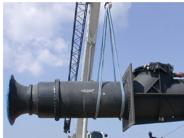
AC-series, Large vertical column pump
