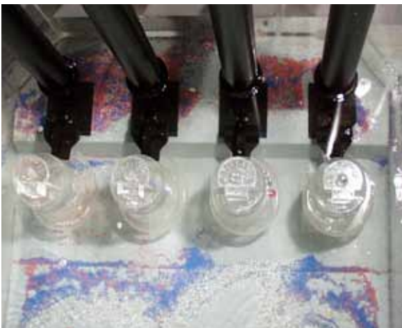
Bottom sediment buildup shown in a scale model test.
