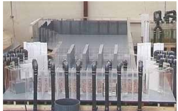
Propeller pump sump design verified by a scale model test.
