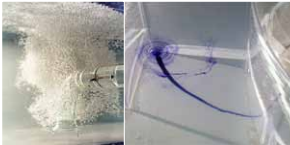
Entrained air and vortex shown in scale model test.
