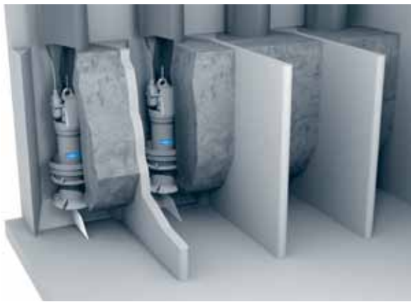
Pump station with formed suction intake in concrete.
