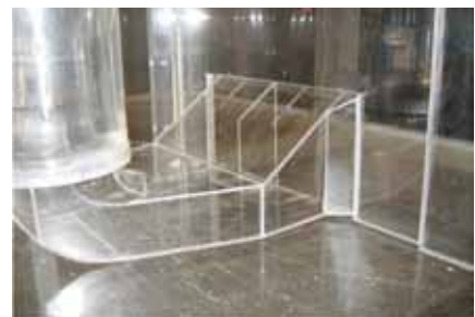
Model of a Flygt Formed Suction Intake device used in the tests.
