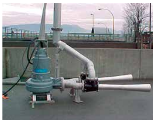
Three Flygt jet aerators JA217 were offered for evaluation by Xylem.
