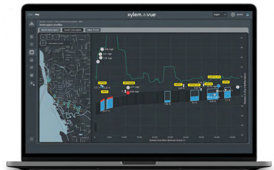
SSO/CSO Prediction and Prevention dashboard showing the available capacity in BSA's major interceptors in real-time, with surcharging, backflow, or overflow warnings.
