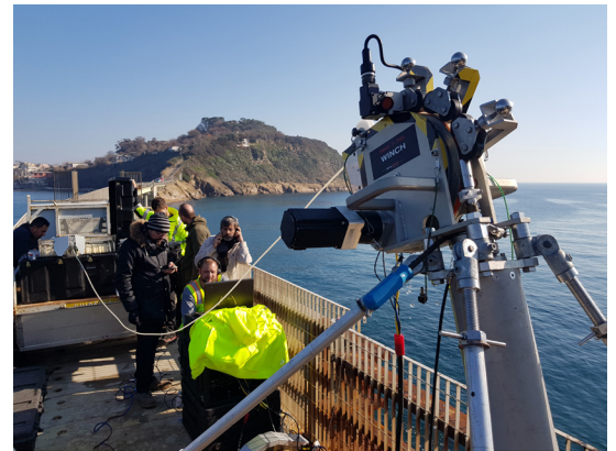
Inspecting the pipelines between Procida and Ischia, Italy with Xylem's Sahara platform.
