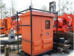
Bypass operations for the Northeast Interceptor Rehab Project included 2 Godwin CD300M Dri-Prime pumpsets with VFD.
