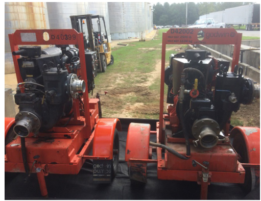
Two of the 10 Godwin diesel-driven CD225M stainless steel pumps, ready for installation for the internal bypass.
