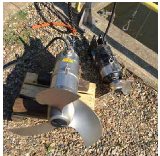
Xylem's Flygt 4220 mixer shown with its predecessor - note the larger more efficient propeller.
