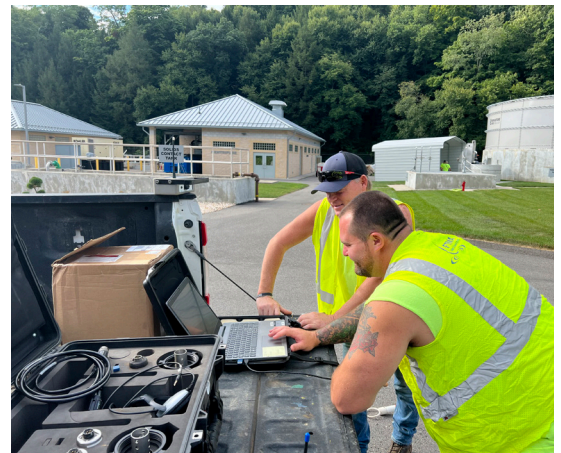
Employees Brandon Carter, Lead Utility Technician (pictured, foreground) and Jim Ervin, Foreman, perform a correlation for a leak based on data provided by Sensus, a Xylem brand's acoustic monitoring solution.
