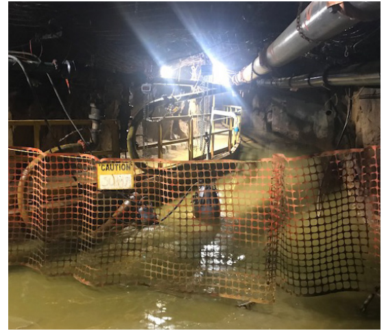
Mine slime is efficiently pumped away thanks to Xylem's broad portfolio of mixer and pumping solutions that combines agitating and transporting liquid out of the sump.
