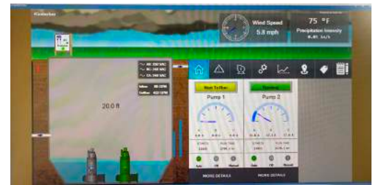
The remote Flygt Cloud SCADA screen at the Kinderlou Lift Station saves Lowndes County time and money by providing them real-time data during a storm event, eliminating the need to send personnel to a site during a storm.
