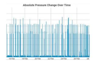
Data from Xylem Water Loss Management solution was analyzed automatically to detect any harmful pressure surges in real time, identify the sources of these pressure surges and their impact on the structural integrity of the pipelines.
