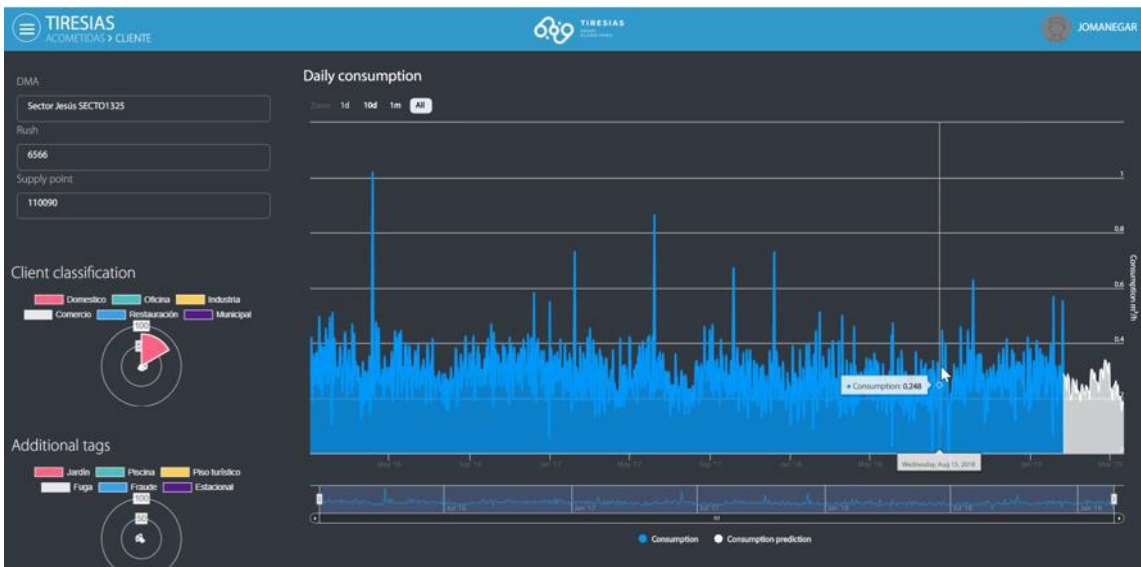
Figure 4.3: Meter-level demand forecast
