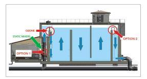
The system design includes two options for dosing hydrogen peroxide. In option 1, peroxide is fed prior to ozone addition to crate hydroxyl radicals in AOP mode. In option 2, peroxide can be used at the end of the contactor to quench any ozone residuals.
