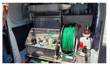
Moosfrei® have over five treatment vans equipped with Flojet's Triplex Series industrial diaphragm pumps, and each pump can be recharged while in transit to eliminate unnecessary downtime.
