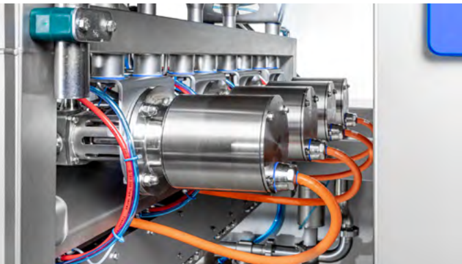
Xylem's Jabsco hygienic flexible impeller pumps push the tomato sauce to the depositing heads at the same rate and speed to maintain equal pressure. As a result, the size of the sauce droplets remain uniform throughout the process.
