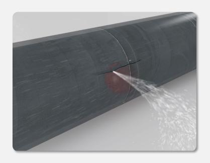
ILI tools can easily identify pipe wall loss, but they fall short at detecting the presence of pinhole leaks. This is where SmartBall steps in.
