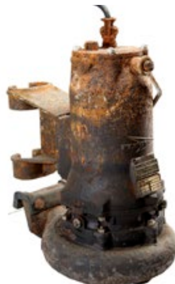
The effects of general corrosion on a wastewater pump that is still functioning after 50 years of use.
