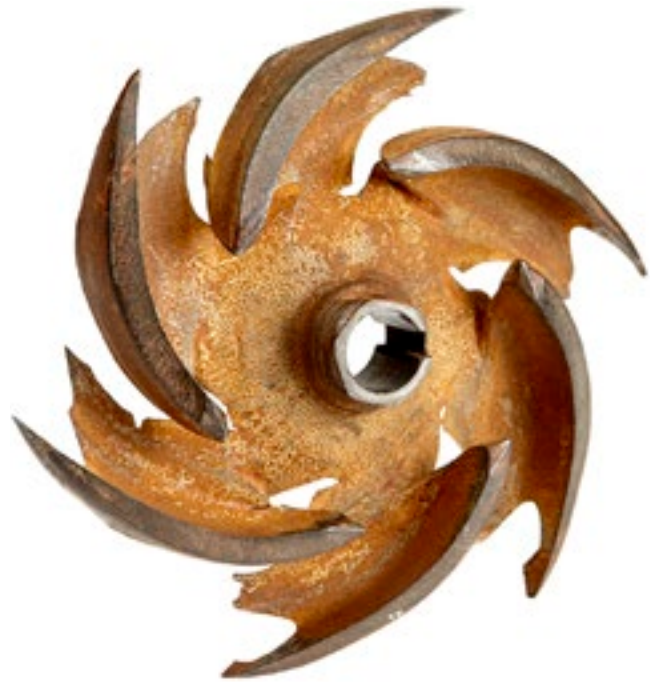
Impeller after an accelerated wear test in a laboratory.
