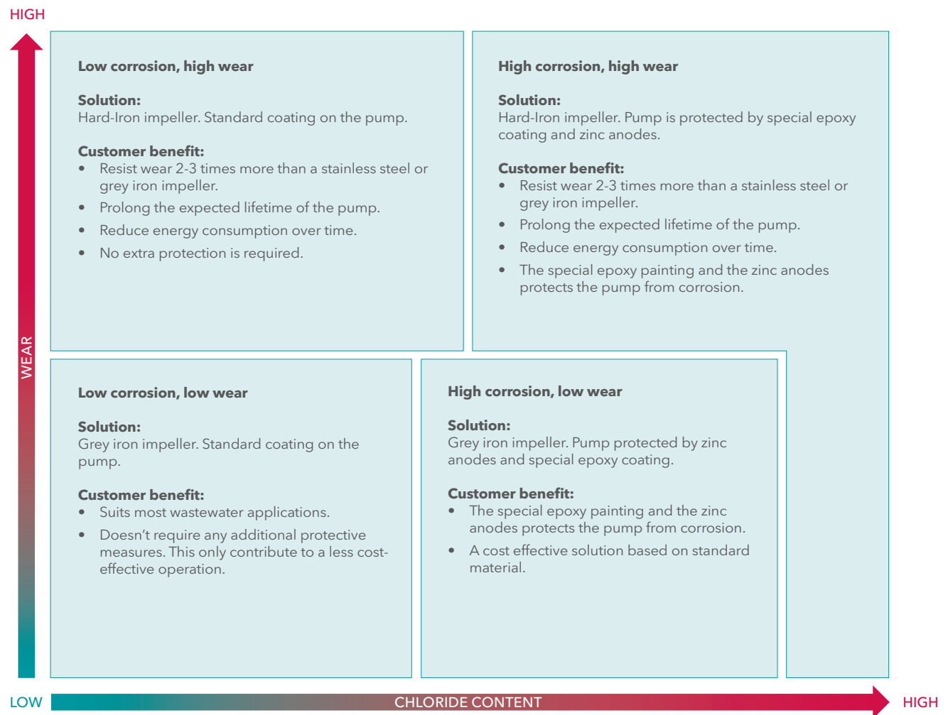
Figure 5: This graph shows recommended impeller materials for grey iron pumps. Other materials may be available but are not recommended for wastewater applications.
