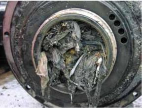
A fully clogged pump is easy to detect (pictured) while a partially clogged pump is rarely detected when a pump is inspected.
